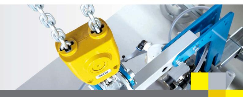
GIS vacuum lifters guarantee the gentle handling of goods of different materials like wood, glass, stone, metal or plastic. Flat, convex and concave shapes with smooth or porous surfaces can be safely, effortlessly and gently transported with the appropriate vacuum lifter.
