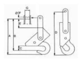
The PIAB IS Hook consists of hook, housing and link. Forged hook, housing and link are of high-grade alloy steel. Unloaded, the spring loaded hook is pulled up against the housing in an open, ready-to-load position where it can easily be hooked onto a sling, lifting eye or other attached hardware.
