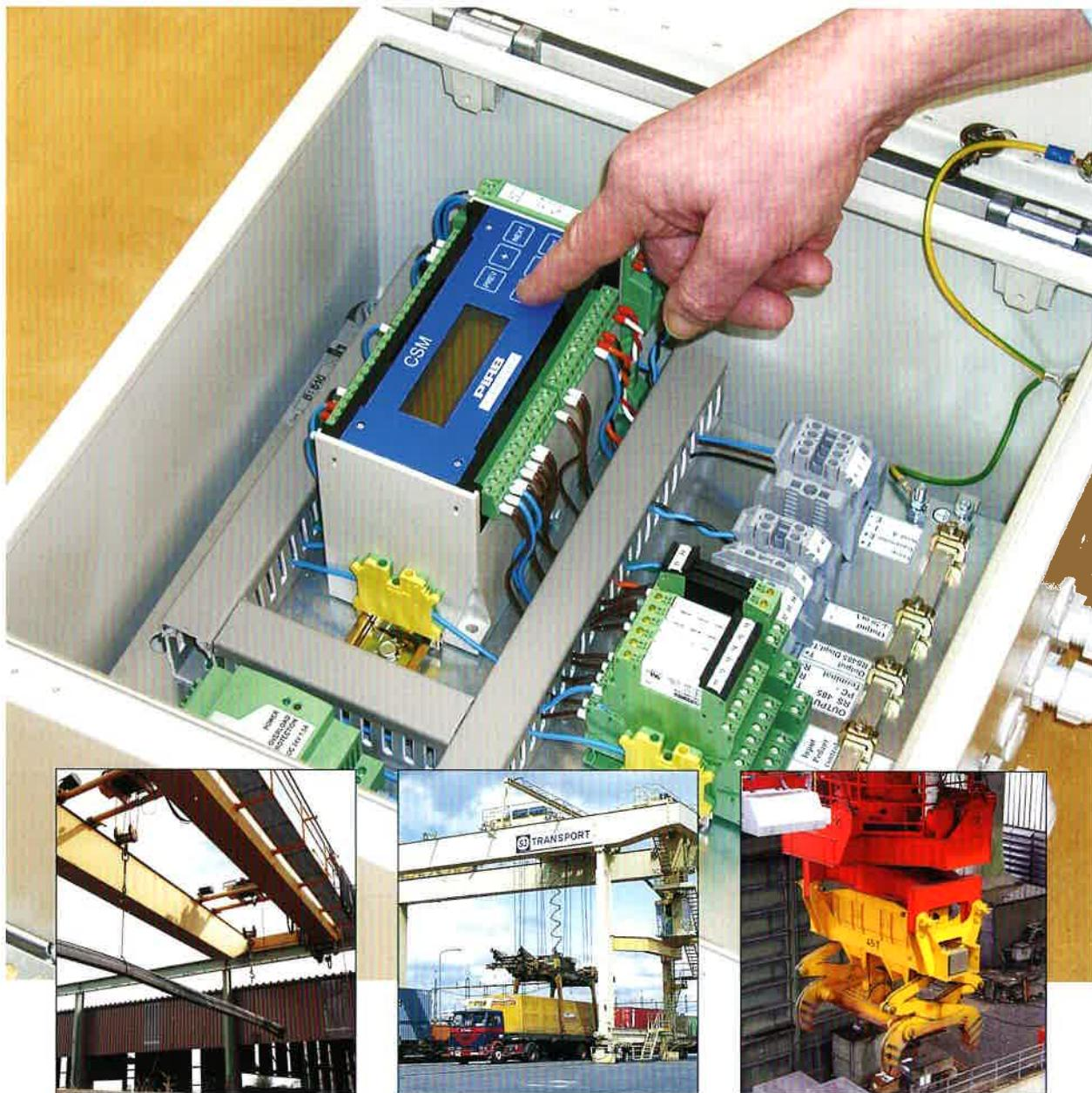
PIAB Crane Safety Monitor (CSM) is an electronic control unit to be used in overload protection systems. The CSM evaluates and computes signals from force transmitters and can be set for alarm at preset alarm limits. By installing the CSM, hazards for personnel and material can be avoided. The CSM will also record the operation of the hoist. The CSM is designed for indoor and outdoor operation in aggressive and demanding industrial environments.
