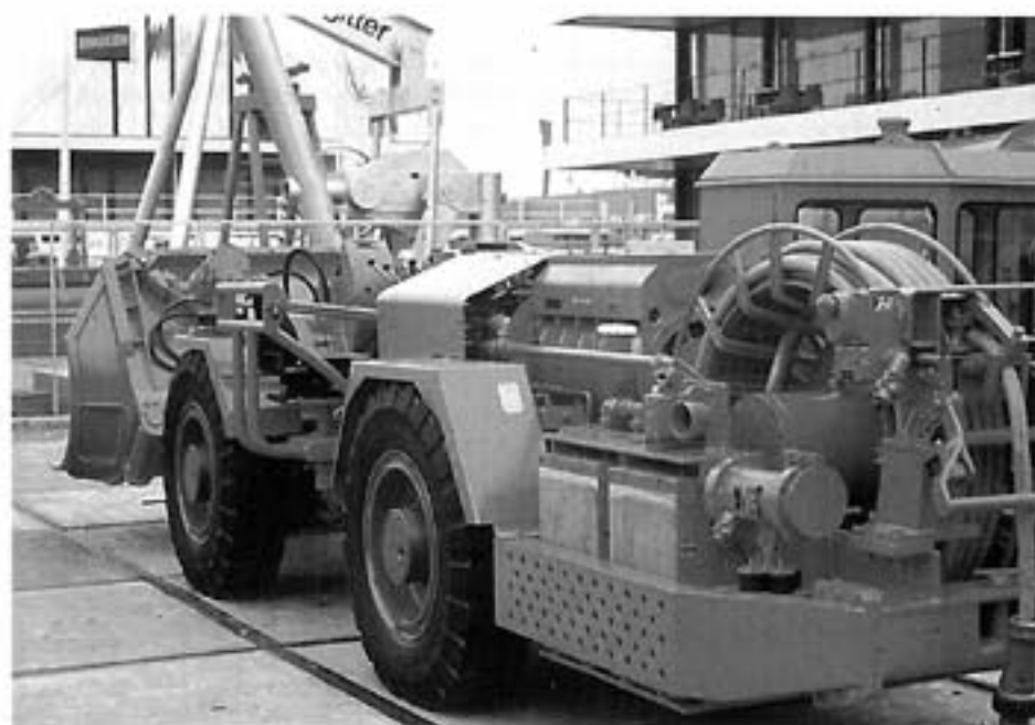
Earth moving machine with EEx slipring assembly
